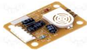
Figure 2.6 SY-HS-220 Humidity Sensor
