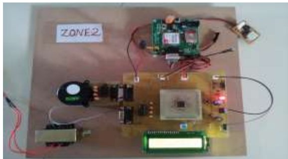
Figure 4.2 Circuit Board for Zone 2
